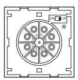
\*Output operation mode is working as Up mode or Down mode according to Up/Down mode selection switch's position.
